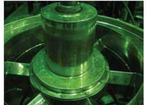
CIP validation by Riboflavin Test
